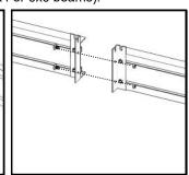
Note: For connecting the base profiles at the corners, x4 **a1** bolts OR hex-head (m6x10) bolts will be used. Each base profile will have one bolt inserted into the top and bottom channel, and then used to secure the anchor legs at the inside corner. Later during the assembly, crop head bolts will be inserted into the top base channel and used to fasten the fixing tabs **m7** to each glazing bar after the panels have been installed.
