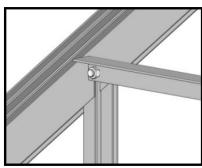
If you temporarily affixed horizontal bar 911 during panel install in Step 2 detach it now; masking tape may be used if needed to hold panels in position.
