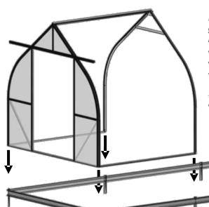
**Note:** This phase of assembly will involve erecting the greenhouse directly on the included aluminum frame. This image is to demonstrate the positioning of the greenhouse on the aluminum frame and you **do not** need to have the Front Gable attached to the A-Frame section via ridgepole and lower sills as shown before attaching it to the aluminum frame.
