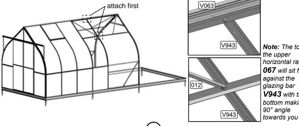
Note: The top of the upper horizontal rail 067 will sit flush against the glazing bar V943 with the bottom making a 90° angle
