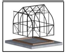
Before securing the aluminum base to your foundation we recommend performing a fit-test. Affix the base pieces in the intended position using the anchor legs, then lay out the lower sills **V913**, **V916**, **V026** (x2), and **V064** (quantity depending on number of extensions in your kit). Ensure that the end troughs of the four anchor legs match both end troughs of side sills and front & rear sills at the same time., as shown in the diagram below.
