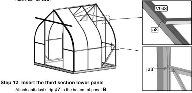
Attach anti-dust strip **p7** to the bottom of panel **B**.
