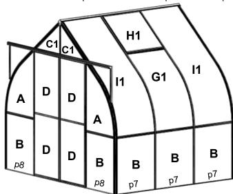
**Tip:** When fitting parts **p6/p7/p8** on the bottom ends of the panels, using a narrow piece of bar soap through the part first will allow them to slide on the panel's edges much easier.
