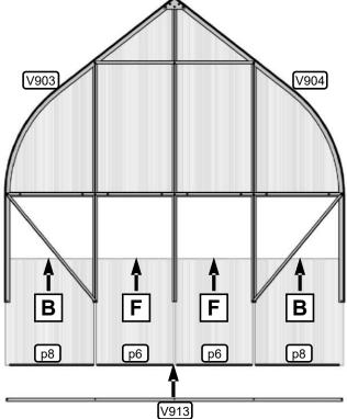
Slide four bolts **a1** each into channel of curved frames **V903** and **V904**. These will be used later during "**Phase 2: Erect Greenhouse**" and may be secured in position with masking tape or nuts **a2** until needed.
