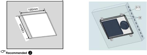
OPTION 2: INSTALL THE FAN USING ALUMINUM SUPPORT STRIPS (may not be included)
