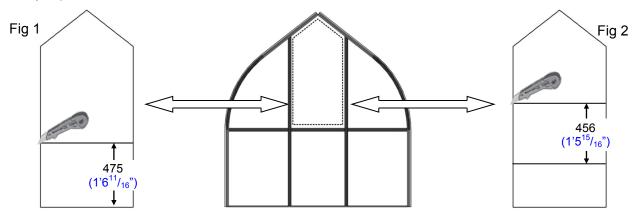
\* Put the PVC anti-dust strip p6 on the end of cutted & remained panel.
